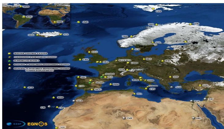
Rys. 1. Segment naziemny systemu EGNOS
