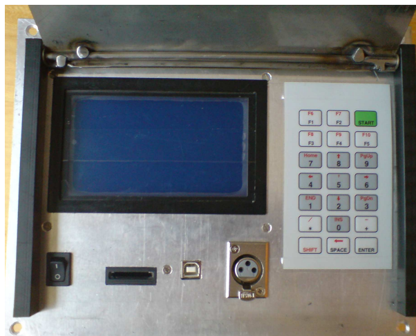
Fig. 1 Device for overhead contact line height and stagger measurement
