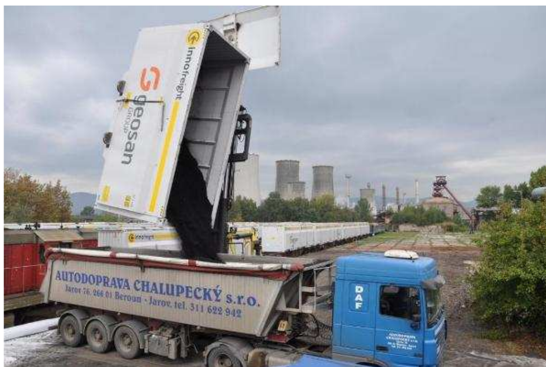
Fig. 12. Emptying of container by rotation by fork lift truck
