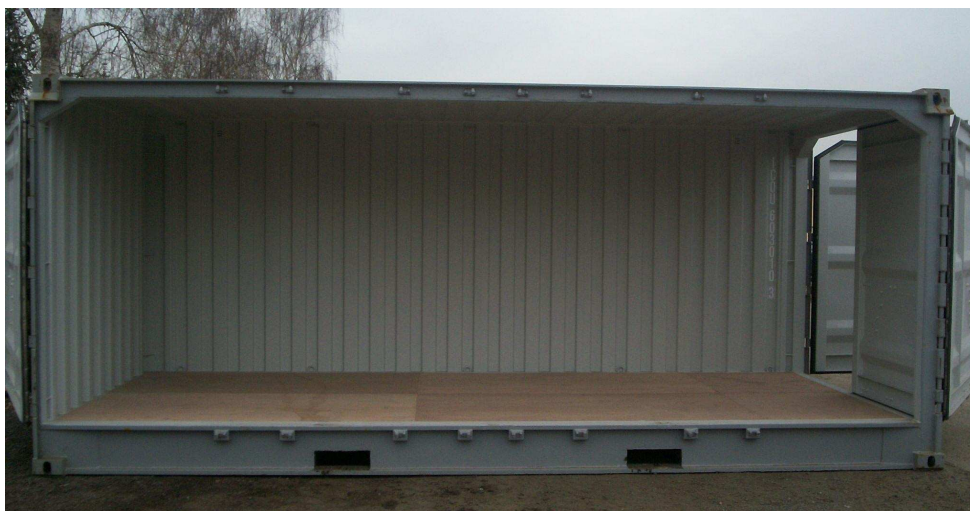
Fig.2. Container equipped with fully opened side wall
