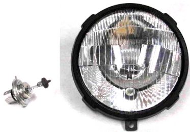
Fig.13. Main light and low beam light reflector of RE03210 (029939) type with H4 light bulb
