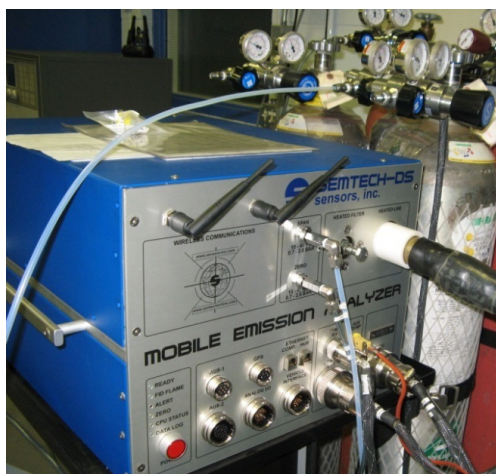
Rys. 2. Analizator spalin SEMTECH DS.
