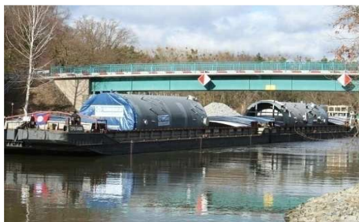
Fig. 5. Transport of pressure reactors with diameter 5,80m for Szczecin-Schwedt refinery
