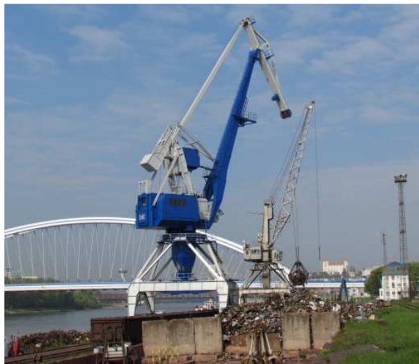
Fig.1. A gantry crane which transfers bulk cargo
