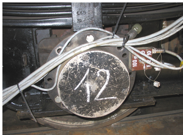
Fig. 2. Measurements of the vibrations accelerations on the axle box of the car
