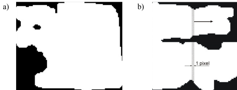
Fig. 4. Images after enlargement: a) image of good sleeper, b) image of bad sleeper along with vertical line using to remove black areas adjacent to horizontal edges of image
