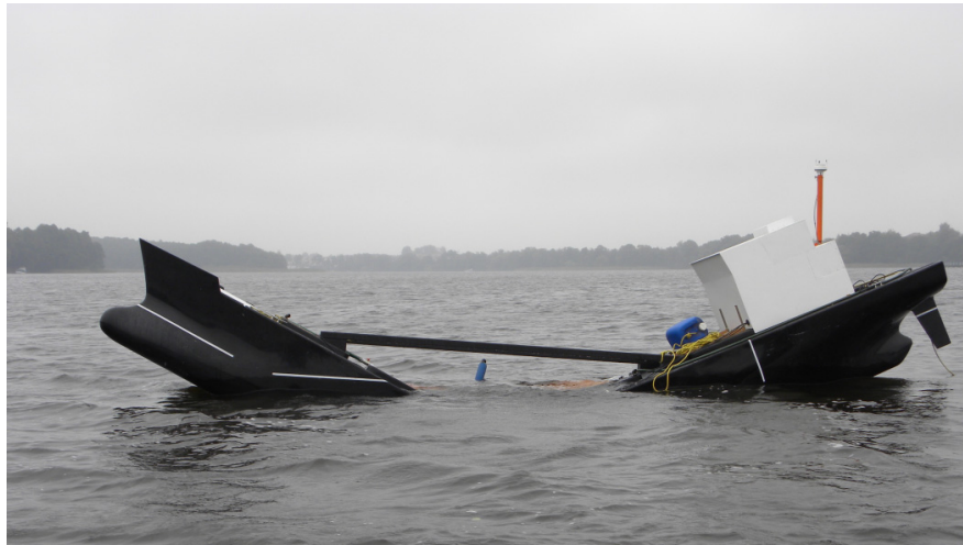
Fig. 3. Drifting model broken in the middle during drift tests
